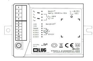
The iBLOC controller has a range of analogue and digital interfaces for controlling the lighting points. Available in the basic version or in a version with a power supply parameter meter. The user can either control the operation of luminaires via the analogue interface (the on/off function with a contactor, controlling light intensity with the 1...10 V protocol) or digitally via the DALI 2.0 interface.
